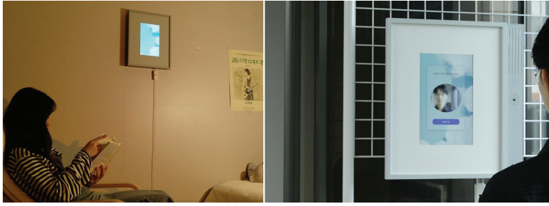
Figure 1. EmotionFrame installed in homes. The device is in idle mode and shows an animated background picture (airplane flying) (left). The cover of Emotion Frame can be physically moved to show mic-camera for self-journaling, and users record their emotional state (right)
